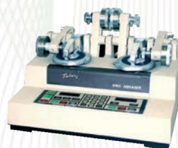
Taber Abrasion Testing Machine
